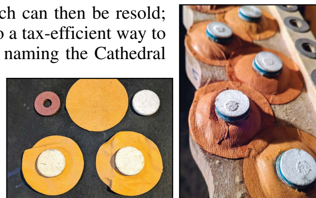
The pouches on the left are new pouches and the pouches on the right are old pouches (these pictures are from a different organ). You can see a crack on one of the pouches on the right which would prevent the note from playing.
